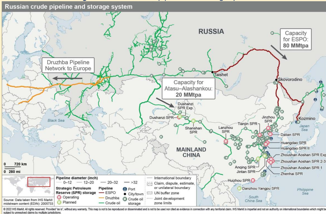
Figure 9: Russian crude pipeline and storage system
